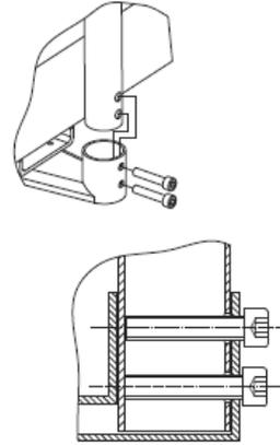
Make sure the direction of the indicator is facing the scale before putting the bolts through to fix the column.
