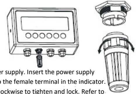
Connect the power supply. Insert the power supply male connector to the female terminal in the indicator. Push and turn it clockwise to tighten and lock. Refer to the image above.
