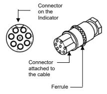
**NOTE:** When moving the scale, take care to prevent bending of the cable and connector too much as over a period of time this can weaken the wires in the connector and cause malfunction.
